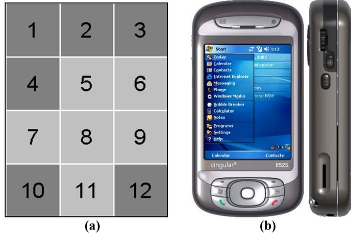
**Figure 38. ThumbSpace Study 1: The input regions shown classified as “hard to reach” in dark gray and “easy to reach” in light gray (a), and an image of the Cingular 8525 used in the study.**
