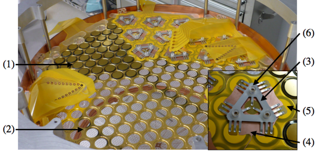
Figure 3.6: Mounted LAAPDs (1) on a gold plated (for improved electrical contact) platter (2). In the inset, platinum plated photo etched phosphor bronze “spider” springs (3) anchor a gang of 7 LAAPDs to the platter while also electrically connecting the copper traces (4) to the flexible cable (5). Acrylic washers (6) prevent the electrical contact between the “spider” and the mounting screws.
