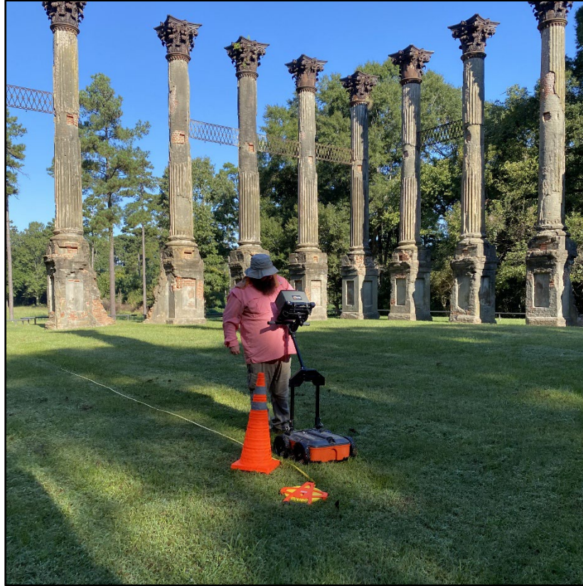
Figure 17: The author calibrates the GPR unit for distance. Image courtesy of Sarah Boone.
