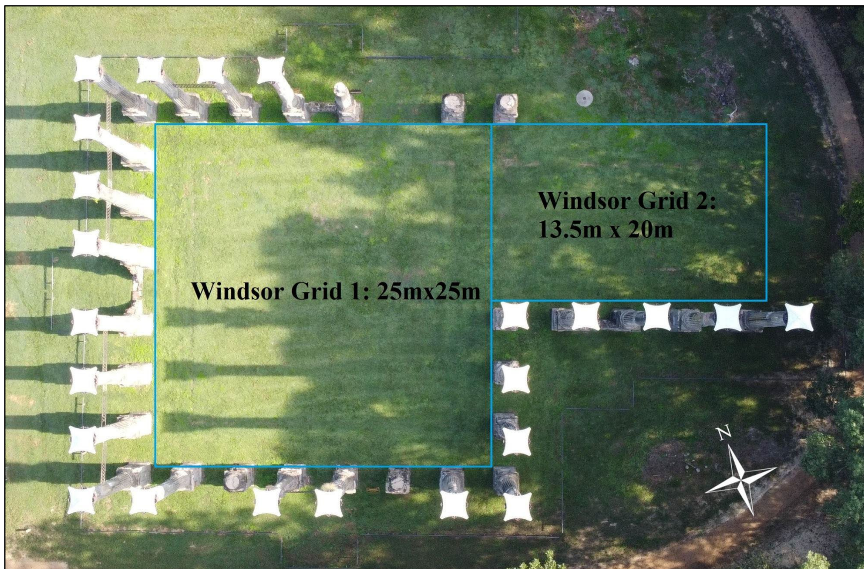
Figure 15: Windsor Ruins survey grids, taken via a DJI Mavic Mini UAV. Image original work of author.
