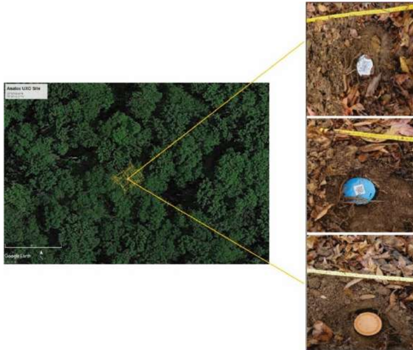
Figure 4.4: Analog UXO Field Site. Pictures on the right show the analog UXO devices made of metal (top), plastic (middle), and ceramic (bottom).
