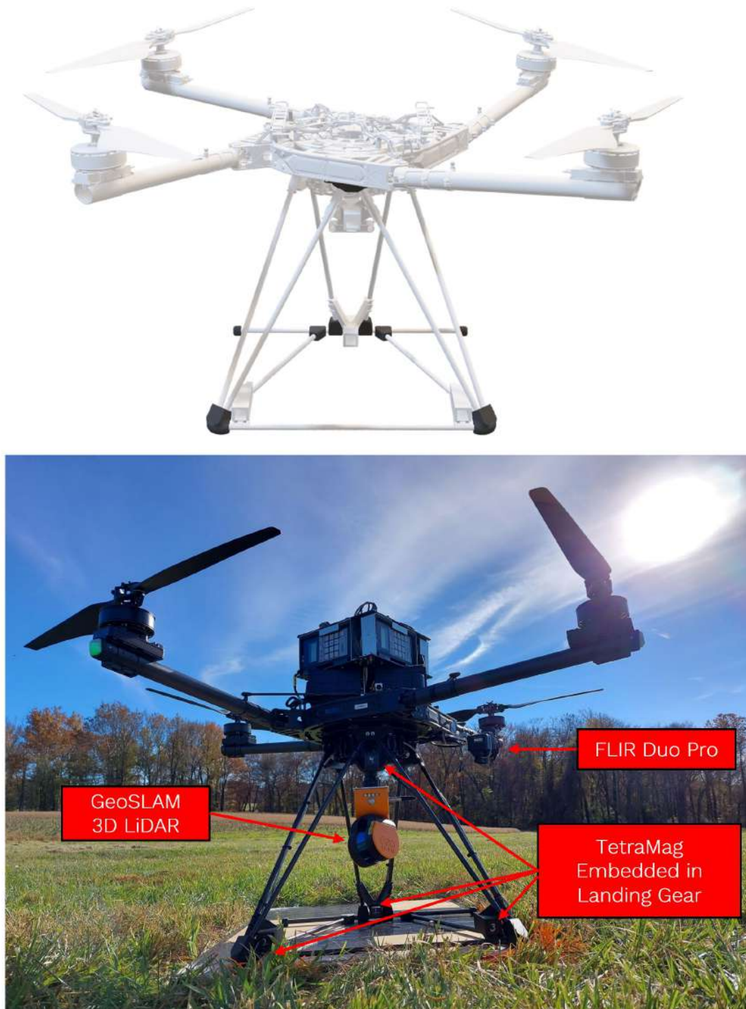
Figure 2.13: Freefly Alta X with integrated drone design (top) and implementation (bottom).
