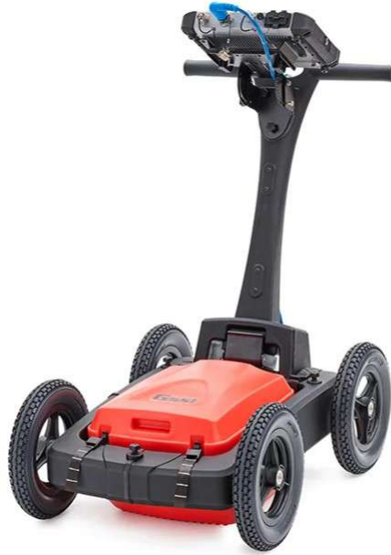
Figure 2.1: GSSI SIR 4000 pushcart with 400 MHz antenna.
