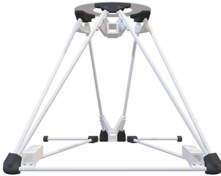
Figure 2.11: TetraMag v2, designed as landing gear for the Freefly Alta X UAV.
