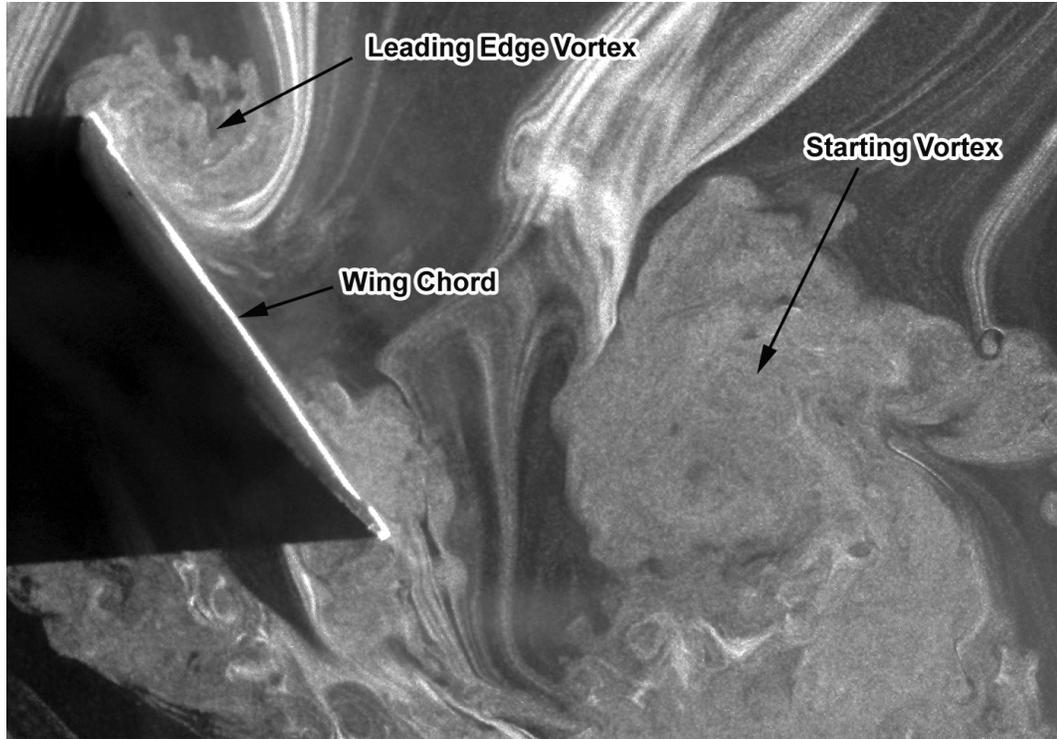
Figure 3.27: Flow visualization image showing the leading edge vortex.
