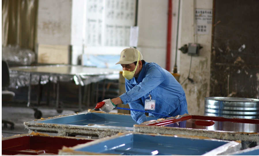
Figure 10: Hand layup process (DOFRP, 2020)
