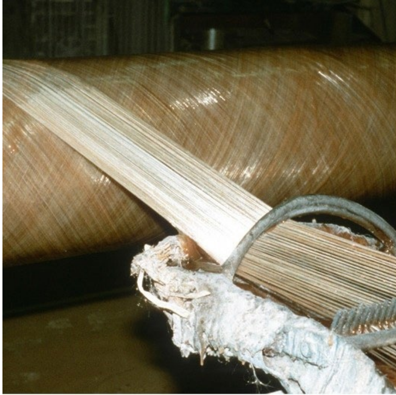
Figure 7: Fiberglass being used in filament winding process (Fibrex FRP Piping Systems, 2020)
