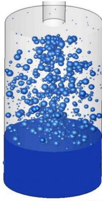
Figure 10: Representative Model of Spray-Droplets in Liquid Piston (Patil et al., 2020b)
