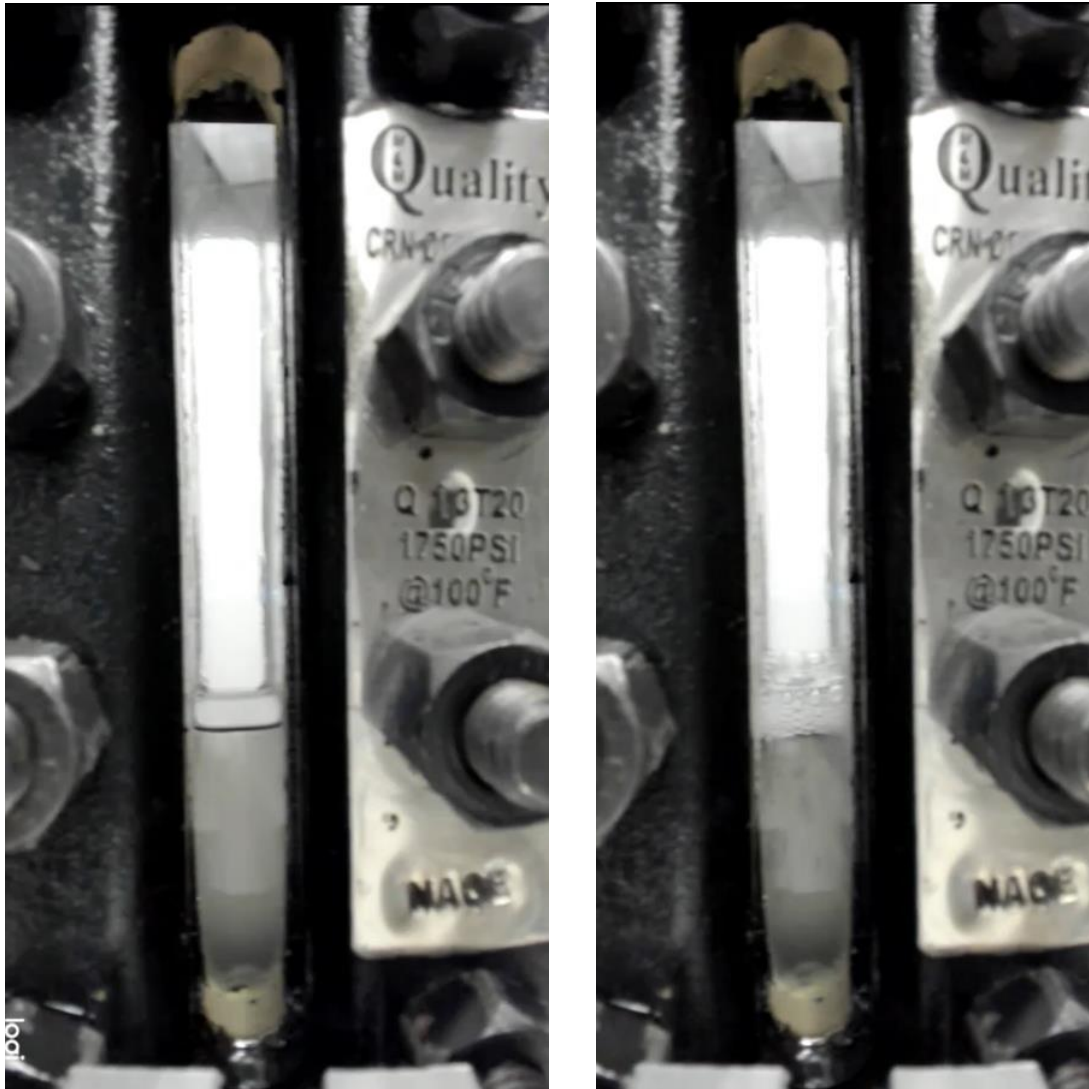
Figure 31: Before (8 MPa left) and After (1.5 MPa right) Picture of Bubbling Occuring
