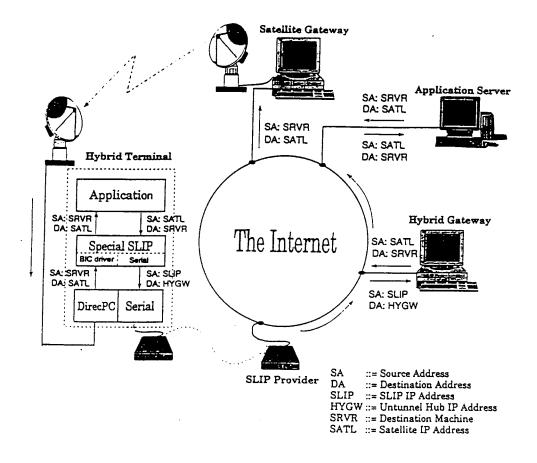
FIGURE 1. Path Traveled by a Tunneled Packet generated by the Hybrid Terminal.
