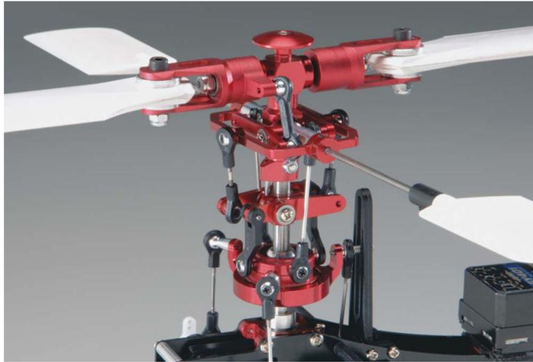
Figure 3.36: Rotor Assembly of an RC Helicopter including Swash plate and negative CP.
