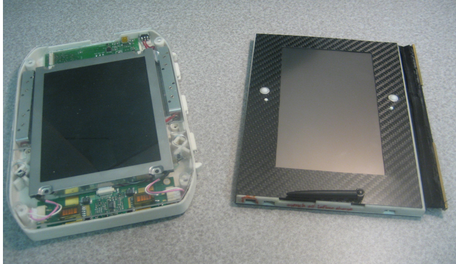
Figure 8 First (left) and second (right) prototypes of the Dual-Display E-book.
