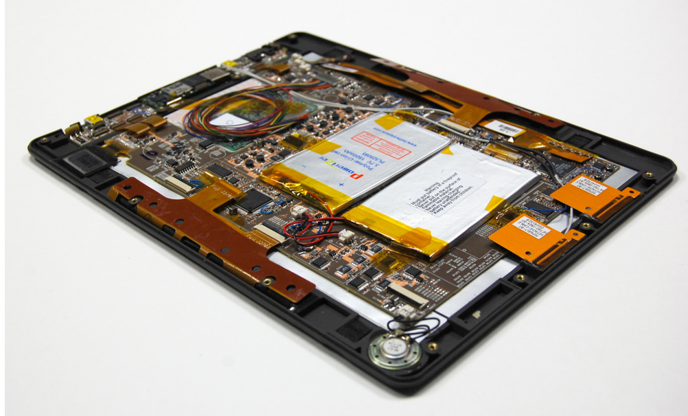
Figure 12 Internal view of the slate device. Note the two flex input boards along the sides and Gumstix carrier board at the top. The orange squares along the bottom edge are the radio antennas.
