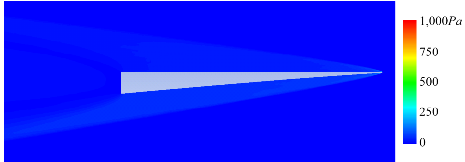
Figure 4.23: Pressure contours for the waverider designed at Mach 6 at a flight condition of Mach 20 and 75k.
