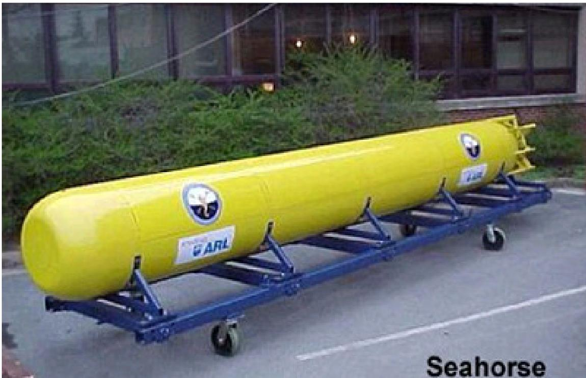
**Figure 1-8: US Navy Seahorse UUV, designed at Penn State ARL.**
