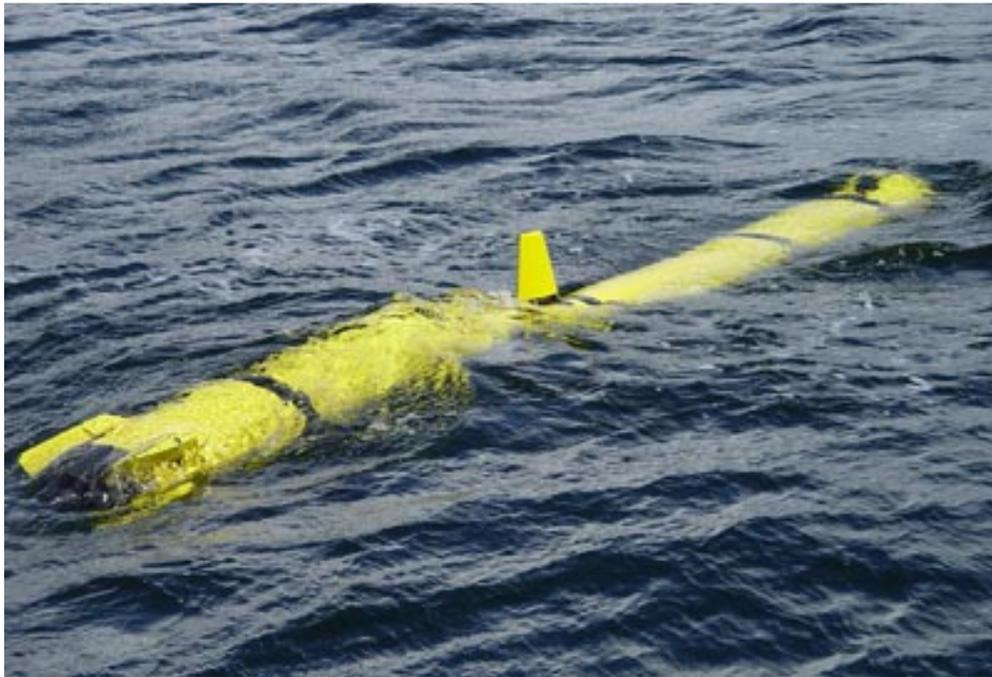
**Figure 1-3: US Navy "MARV" battery powered UUV [7].**
