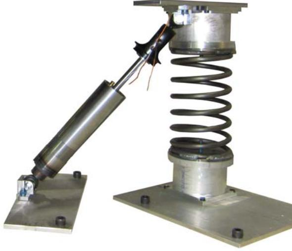
Figure 4.2: Single suspension leg.
