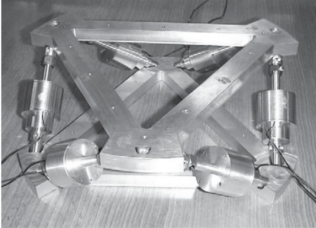
Figure 1.14: Cubic hexapod manipulator with piezoelectric actuators [36].
