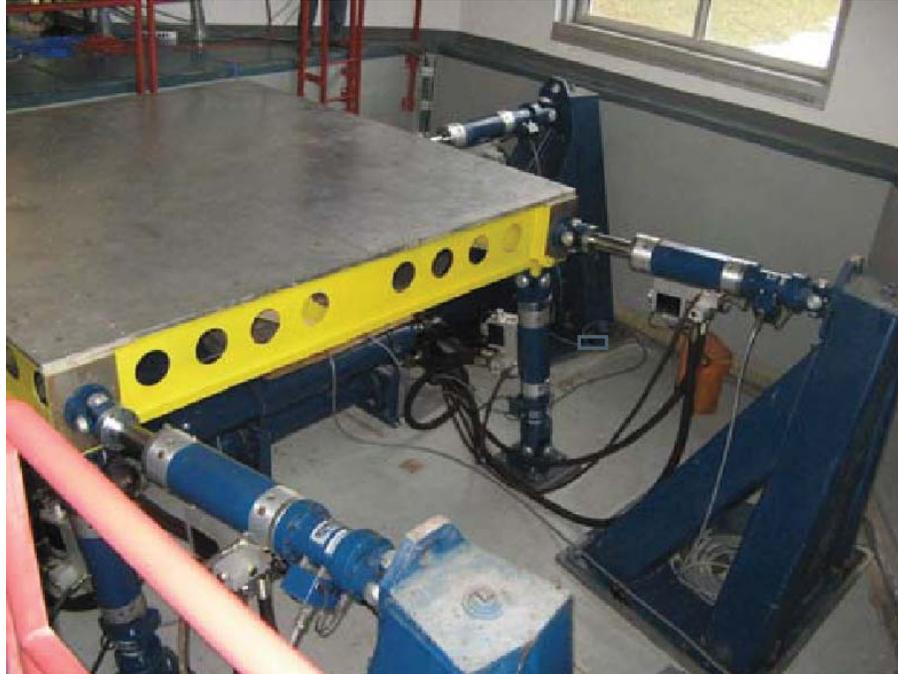
Figure 5.19: GW-NSF hydraulic shake table at George Washington University.
