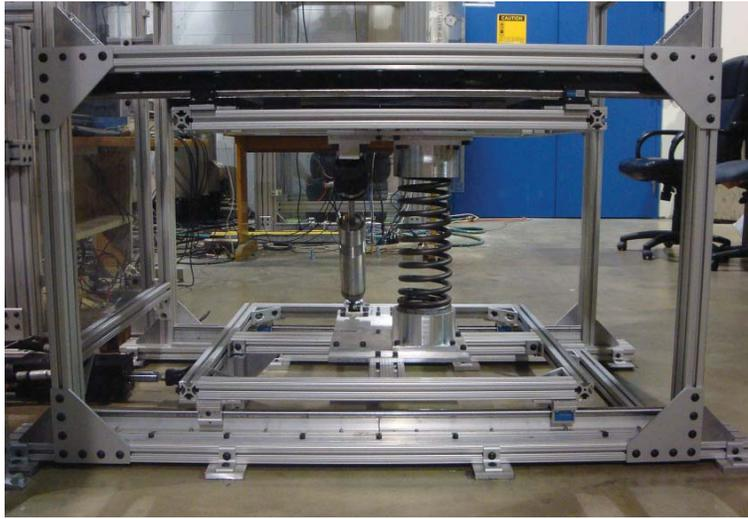
Figure 5.9: Lateral 1-DOF shake table test stand.
