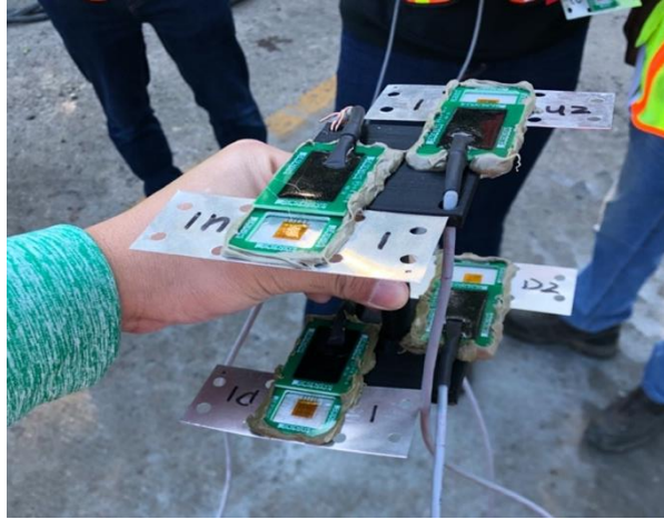
Figure 6-7 Customized sets of strain sensors
