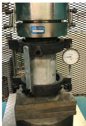
Figure 4-4 Compressive strength or Young's modulus test setup
