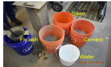
Figure 4-3 ECC lab mixes at the NRMCA's Lab in Greenbelt, MD
