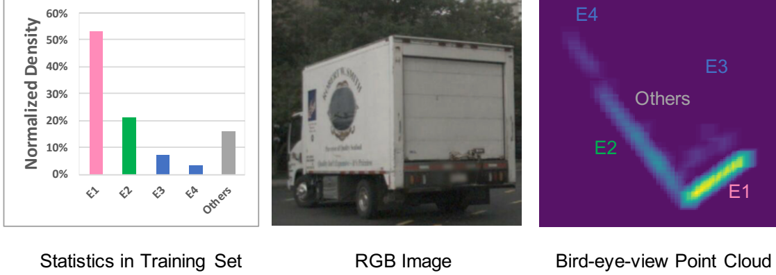
Figure 2.1: Left: we calculate the average point density across different parts of objects in BEV of nuScenes training set. E1-E4 indicate four edges sorted by their normalized density scores (sum to 100%) and others denotes areas inside objects. We set each edge width as 10% of the length along the object size and only objects over more than 100 points are counted. Middle and right: we visualize an example of the LiDAR point cloud in 2D image and its corresponding bird’s eye view (BEV). Clearly, most of the point clouds locate on the contour of the object
