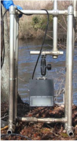
Figure 2.2: The Dual Frequency Identification Sonar Unit (DIDSON) for generation of fish count. Panel A is an image of the DIDSON device before its deployment in a shallow river system (a picture courtesy of SERC). Panel B is a screen capture of a DIDSON video where a river herring can be seen passing by (image credit: Sinclair, 2013).
