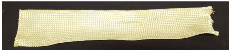
(c) Kevlar braid used in FAM construction
