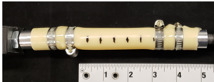
Figure 6.14: Latex bladder tensile test specimen
