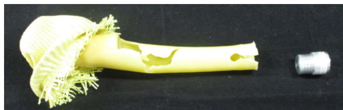
(c) Failed FAM with braid rolled back to expose bladder
