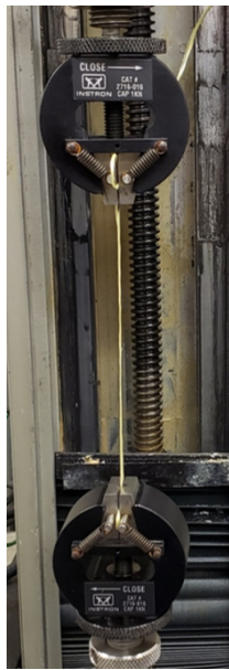
(a) Single thread tested on Instron machine
