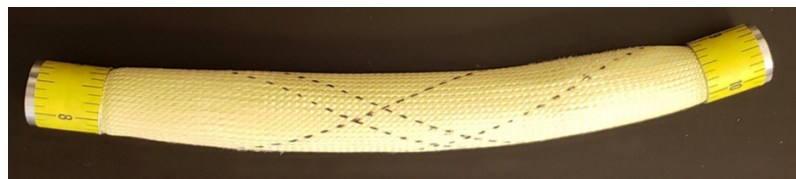
(b) FAM threads marked for measurement of N and B_0
