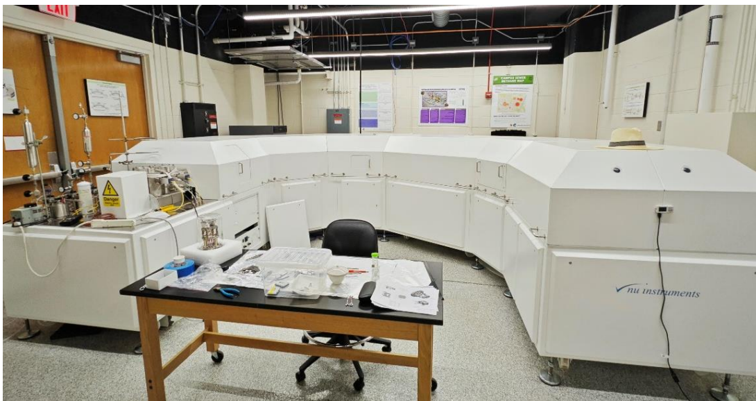
Figure 2.9. Photo of the Panorama mass spectrometer housed at University of Maryland. Photo taken by Jiayang Sun. Except for the sample loading section on the far left, the rest part of the mass spectrometer is covered by metal shields to maintain temperature stability and prevent dust. Unshielded photos are not shown to avoid any patent disclosure conflicts.
