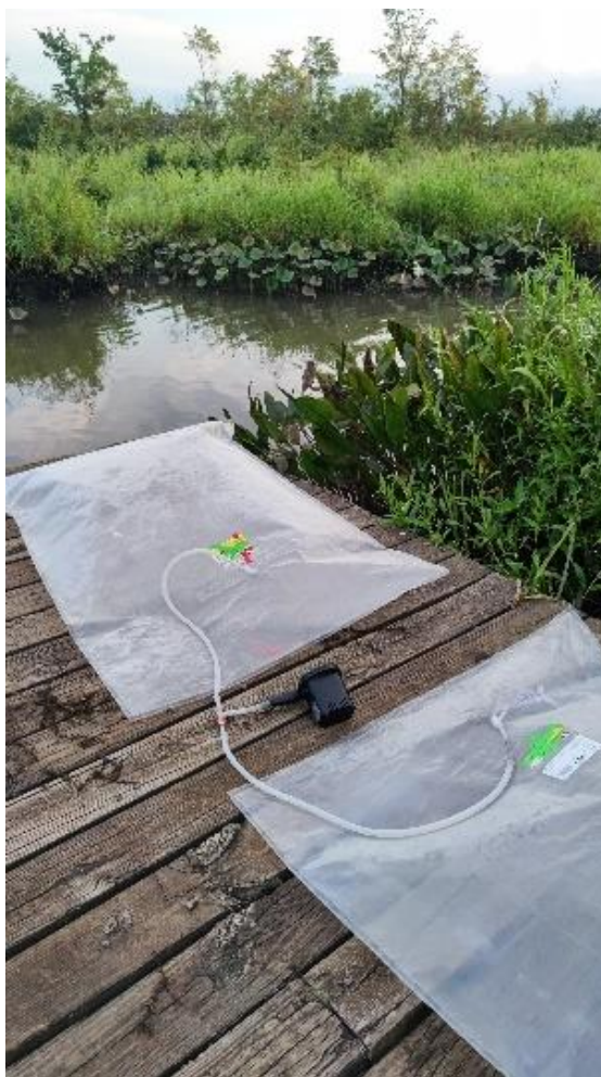
Figure 2.2. Using one mattress pump to fill 2 * 200L Tedlar bags simultaneously. Photo taken by Jiayang Sun on September 3, 2022, at 6:53 AM at Jug Bay Car Boat Launch (38.811565, -76.710501).
