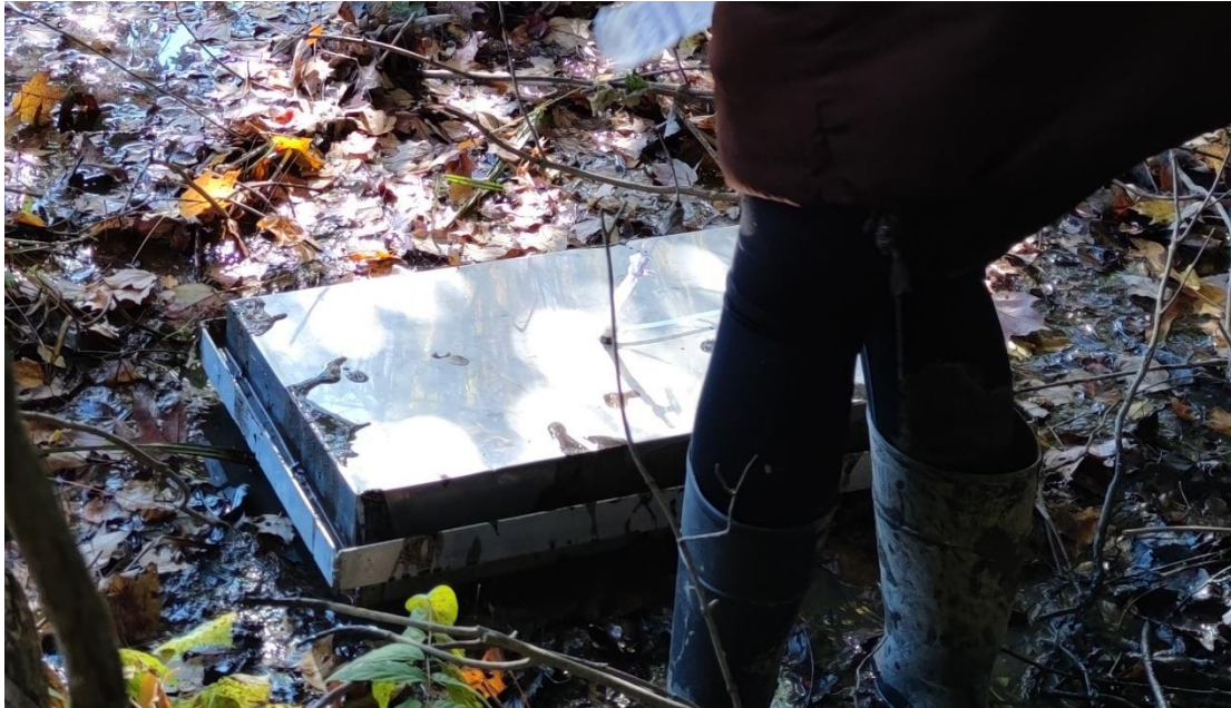
Figure 2.3. Photo of a chamber sampling from wetland. Photo taken by Jiayang Sun on November 05, 2021 at noon, at University of Maryland Golf Course (38.996084, -76.955649).
