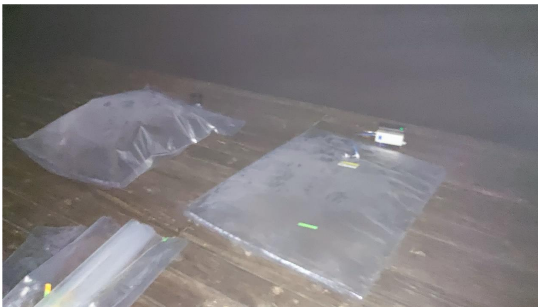
Figure C.2. A closer view of the sampling bags and the pump. The photo was taken on November 4, 2022, at 6:43 AM. Two sampling bags are simultaneously being inflated by two portable pumps to collect air samples. Dense fog was present.
