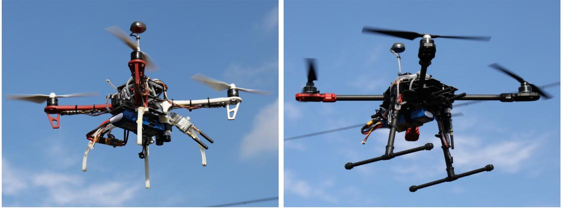
Figure 5.8: Quadrotors in the testbed with the DJI F450 frame (left) and the Tarot 650 frame (right)
