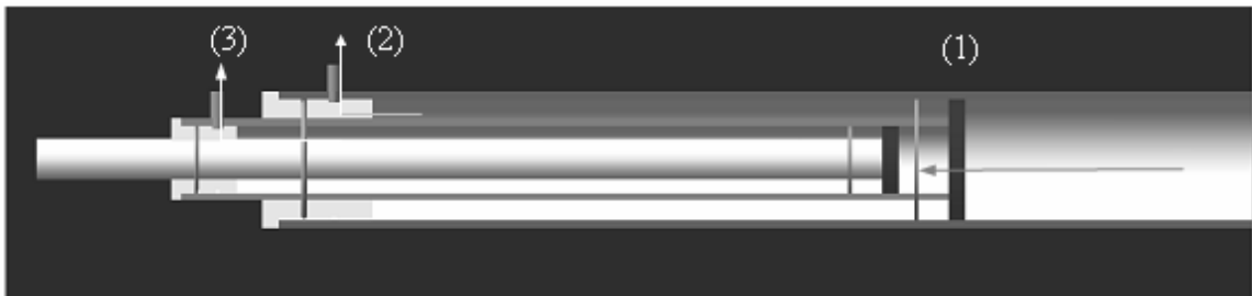
Figure 23: Telescopic spar and input/ output control valves
