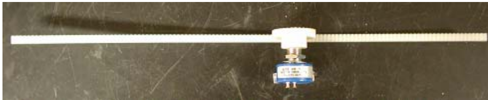
Figure 64: Pinion Mounted on the potentiometer
