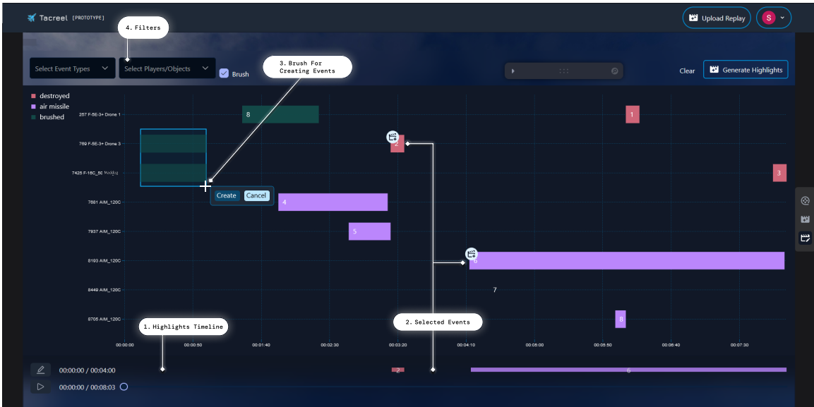
Figure 5.6: Director tool with event timeline. The timeline is organized with units on the vertical (Y axis) and time on the horizontal (X axis). Colored boxes represent events detected by the rule engine. Users can create custom events by brushing the timeline.
