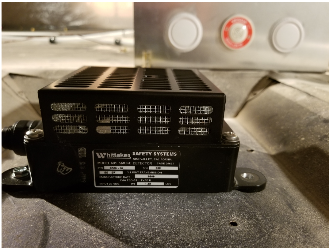
Figure A.9: Whittaker photoelectric spot detector.
