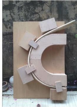
2. Place malleable stripped bamboo into mold to curve to hold shape
