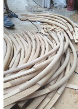
3. Take stripped bamboo out of mold and refine until bamboo is smooth
