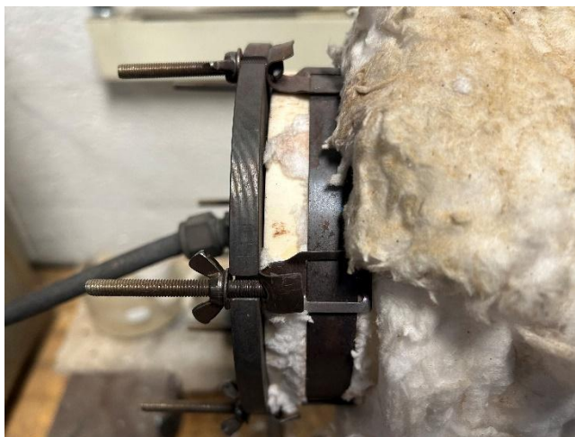
Figure 23: A small gap between the endcaps and the tube furnace was present after pyrolysis.
