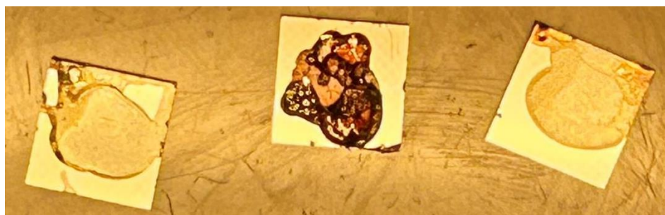
Figure 13: Polymer films created from 0.33g/mL, 0.4g/mL, and 0.2g/mL mixtures, presented from right to left.
