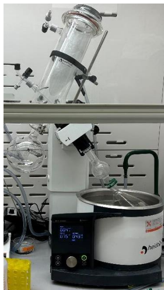
Figure 6: A rotary evaporator quickened the removal of solvent due to liquid films evaporating at increased rates as the flask is rotated in a warm pool of water.
