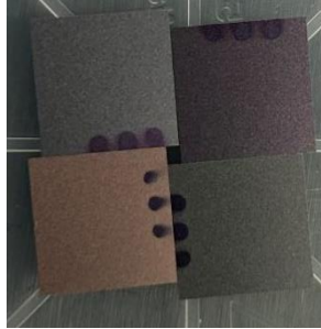
Figure 19: 50 nm of nickel (top left), 20 nm of nickel (top right), 40 nm of iron (bottom right), and 200 nm of copper sputtered onto diamond surfaces.
