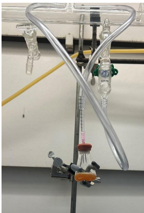
Figure 3: Bromoform dried over calcium chloride while being purged under nitrogen.
