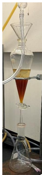
Figure 8: The separatory funnel allowed for fluid extraction based on density differences.
