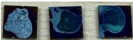
Figure 22: The first batch of polymer films degrading after annealing in the tube furnace.
