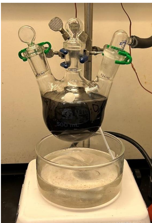
Figure 5: The solution of sodium, THF, and naphthalene turned dark green after mixing for two hours.
