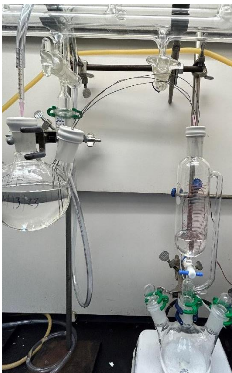
Figure 4: Dry THF transferred between flasks using cannulas and an addition funnel.
