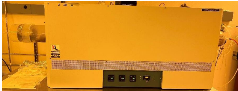
Figure 20: The first annealing tests were conducted for metal-on-diamond chips using this tube furnace at the Nanocenter.
