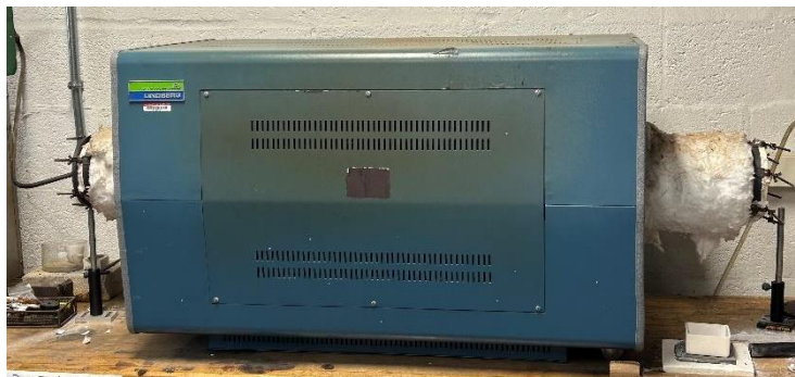
Figure 15: A tube furnace with metal endcaps was first used for long term pyrolysis.
