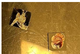
Figure 14: Film deposition from the synthesized homogeneous 0.33g/mL solution (left) and the 0.2g/mL solution (right) created using the polymer obtained from National Polymer.
