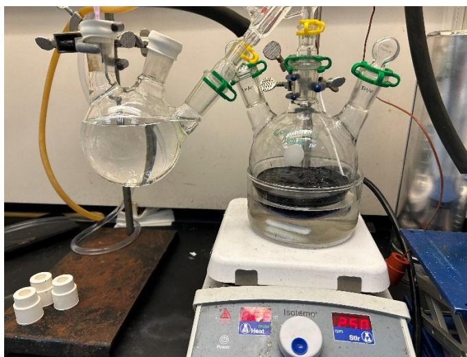
Figure 2: THF distilled into the 500 mL 3NRBF after the mixture turned dark purple.
