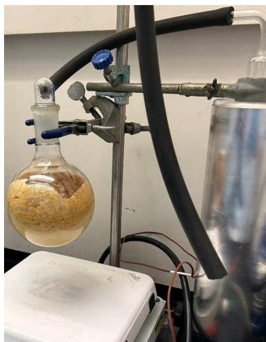
Figure 7: The solid residue was evaporated to dryness using a vacuum pump. A cryotrap froze solvents before reaching the pump.
