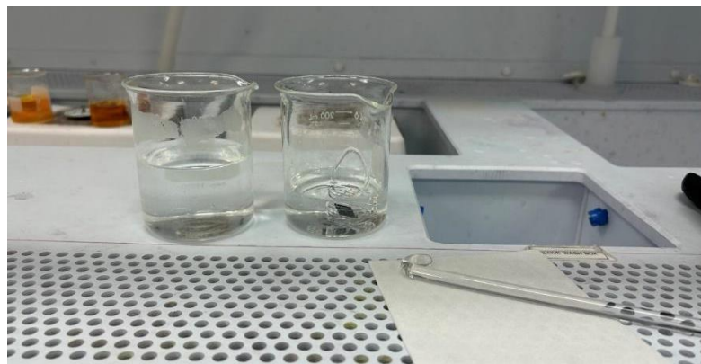
Figure 18: A glass bucket was used to immerse the diamond-on-silicon chips into the 3:1 sulfuric acid to nitric acid solution.
