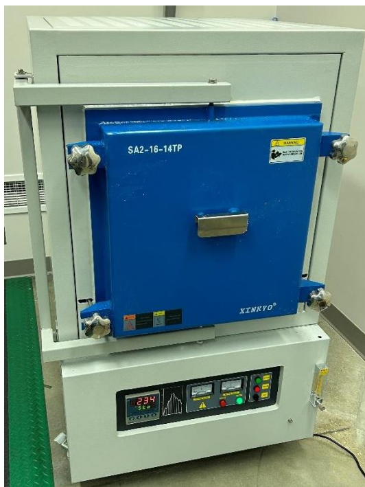
Figure 16: A sintering furnace with metal endcaps was used for long term pyrolysis for the second batch of films.
