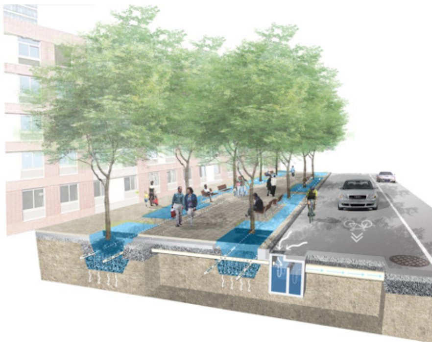
Figure 141: Image of Underground Stormwater Detention
