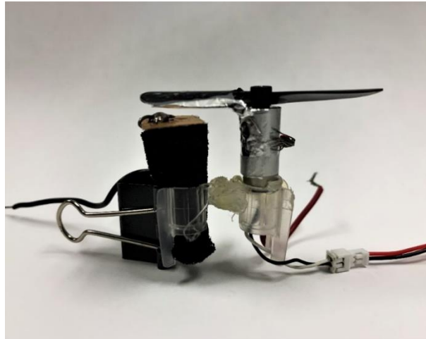
Figure 5.13. Photo of assembled propeller variable capacitor prototype with aluminum foil sleeve electrode over propeller and motor.
