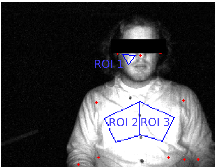
Fig. 1 Labelled ROIs from Camera Feed. ROI 1 denotes the subject’s cheek, and ROIs 2 and 3 cover the subject’s lungs
