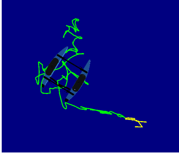
Figure 5.3: In the simulation environment, the ArduPilot properly rotates the boat in-place.
