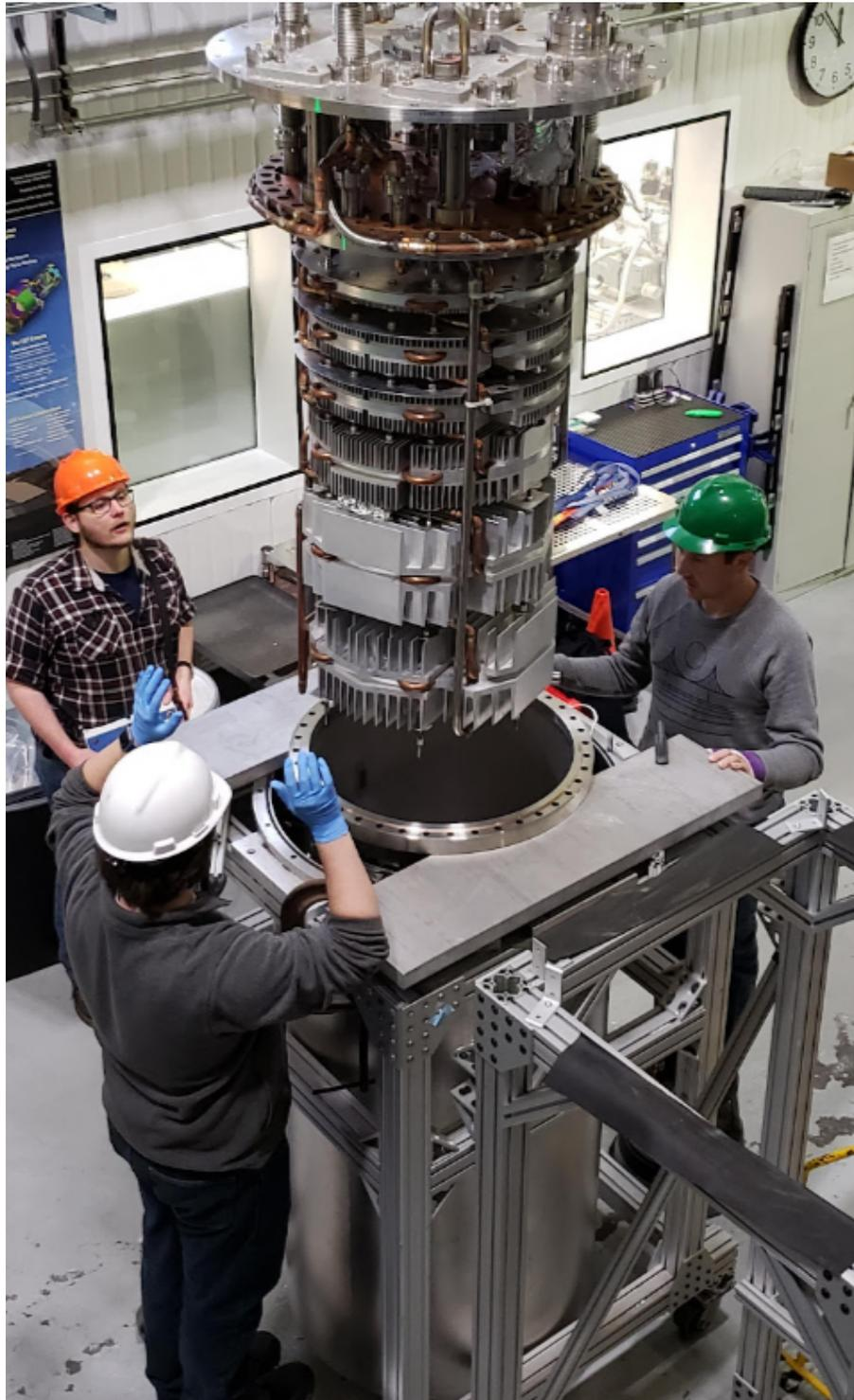
Figure 5.4: Lowering the krypton removal freezer into the freezer vessel. As the helium-xenon mixture passes through the freezer, xenon ice forms on the aluminum fins. Aluminum plates are thermally coupled to copper tubes flushed with liquid nitrogen. Heaters and temperature sensors on each aluminum plate control the temperature.
