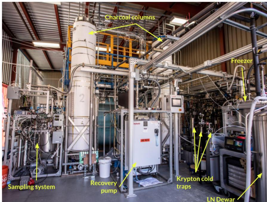
Figure 5.2: An image of the krypton removal system at SLAC. The system is in a metal structure, semi-exposed to the outdoors. Not shown here are the helium re-circulation pump and fluitron compressor. This image is taken from reference [28].
