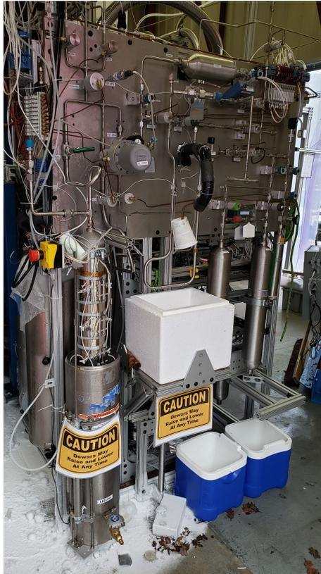
Figure 4.21: A picture of the mixing panel, sniffer, and recovery bottle. Additional components that supported operations of the SLAC XPM are installed with the mixing panel on the side of the SSS.
