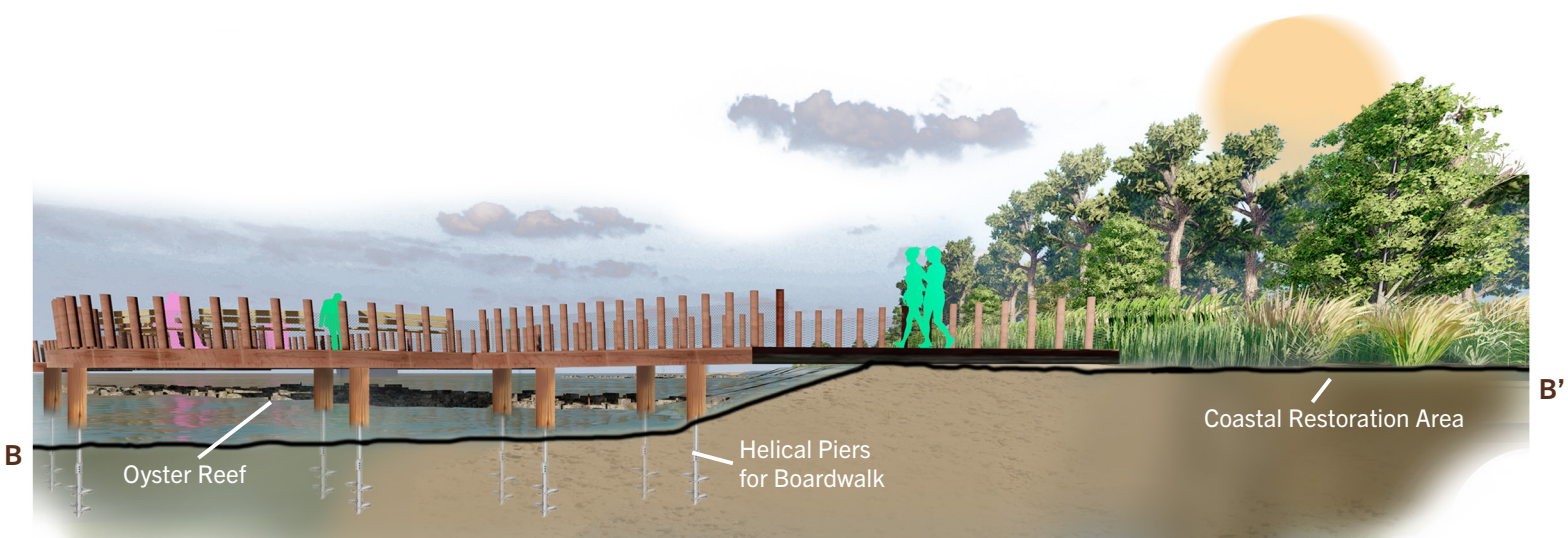
Figure 85: Section Through the Boardwalk and Restoration Area
