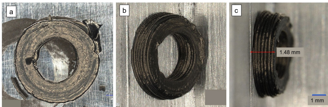
Figure 5.2: (a) top view (b) 45° (c) side views of printed permalloy toroids after drying. The toroid shape is regular, and the layers are distinct.
