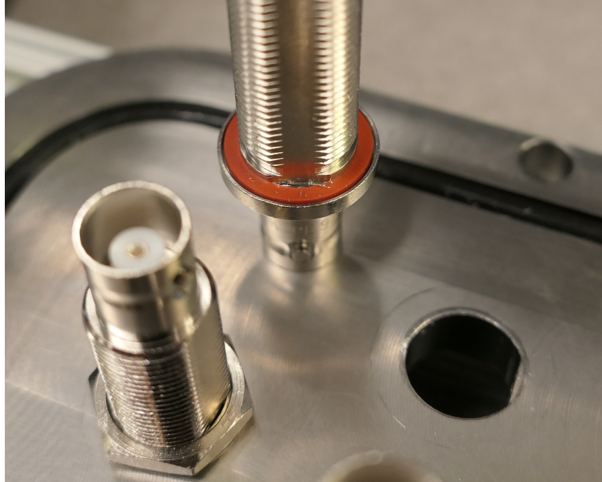
Figure 4.39.: Pieces of metal were observed on the sealing face of an o-ring (orange) belonging to a leaking feedthrough. The metal was believed to originate from threads on the feedthrough, which was likely overtightened. At the bottom left, a feedthrough as it was normally installed can be seen.
