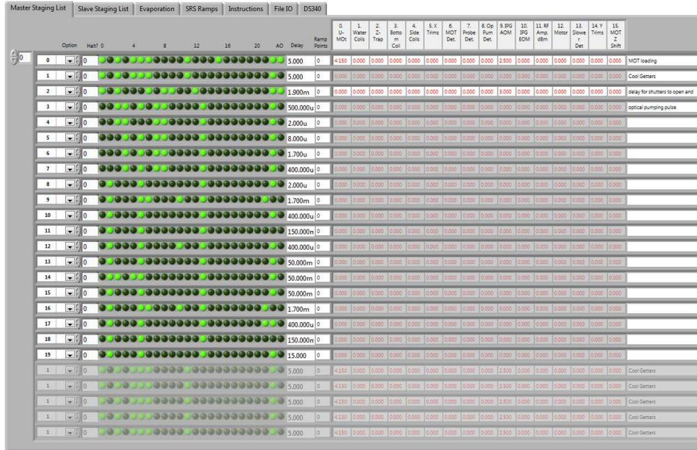
Figure 3.14: Graphical user interface for the software controlling the apparatus. Green circles represent digital outputs, while red numbers are analog outputs. Each set of outputs is held for the amount of time in the “delay” column.
