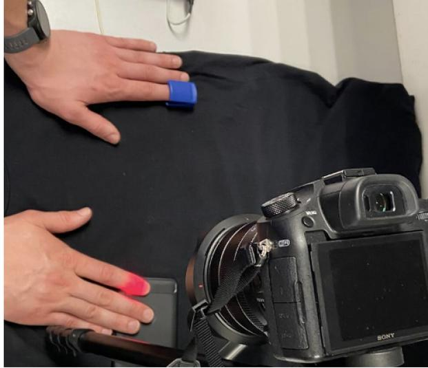
Figure 2.6: Experimental setup with ground truth recording on the left forefinger, a smartphone light behind the right forefinger, and the camera collecting data over a plain background.
