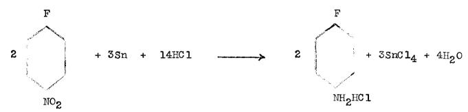
means of tin and hydrochloric acid (64). Add 75 Gm. of tin to 37 Gm. of p-nitrofluorobenzene in a three-necked flask fitted with a reflux condenser, mechanical stirrer and a dropping funnel. Add slowly, from the funnel, 150 cc. of hydrochloric acid with constant stirring, cooling the flask when the mixture becomes too warm. After complete addition of the acid (about one hour), reflux the mixture for 30 minutes and allow to
