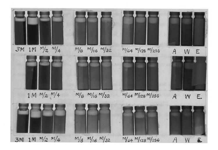
The tubes in the top row contain dilutions of sec-butyl iodide; those in the middle row, n-heptyl iodide; and those in the bottom row, iodobenzene, in the strengths shown. The last three tubes in each row contain alcohol (A), water (W) and an empty tube (E).
