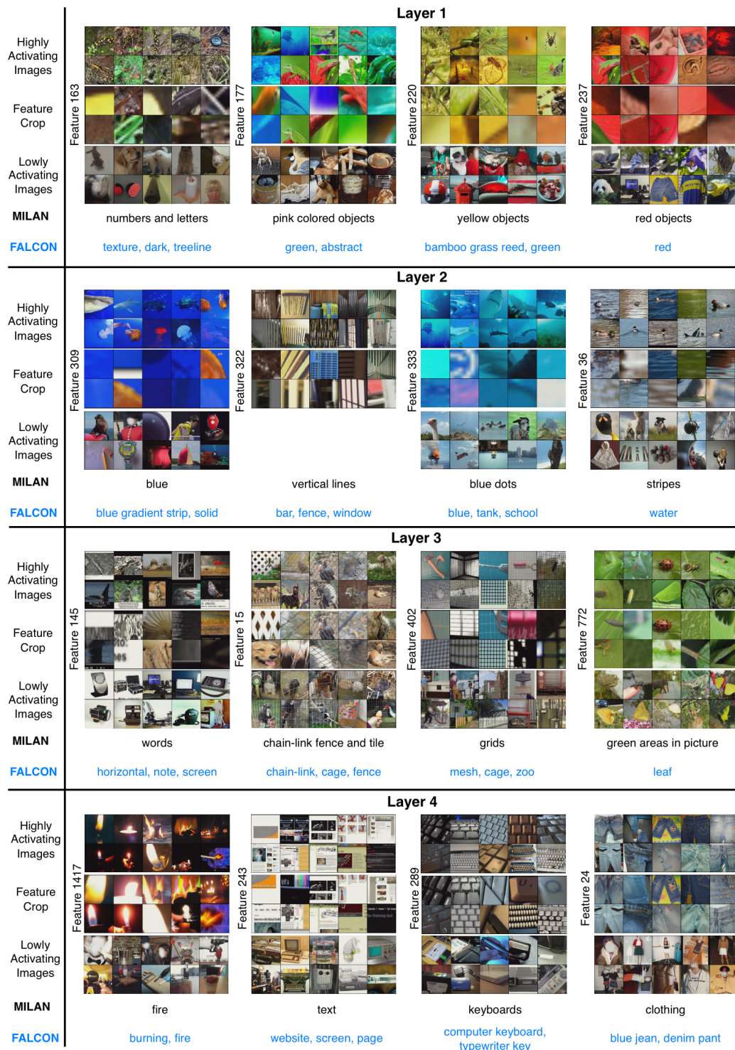
Figure B.8: Concepts for features of various layers of supervised ResNet-50: We extract concepts from random features of layers of supervised pre-trained ResNet-50. We compare FALCON concepts with MILAN concepts.
