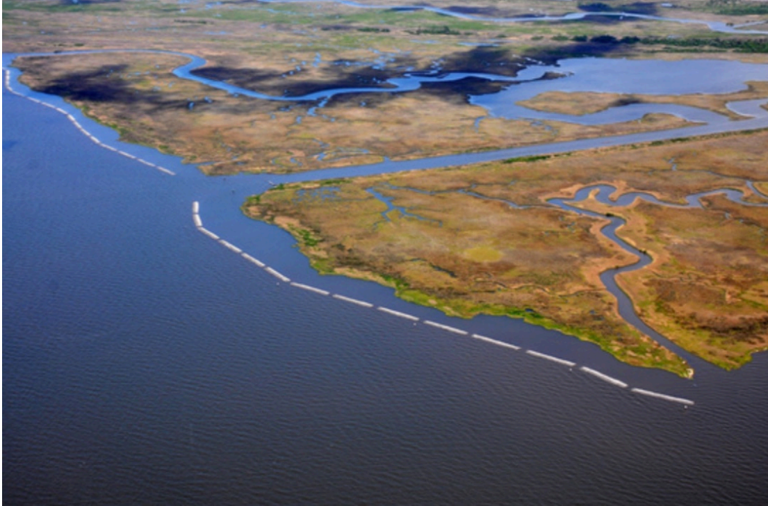
Fig. 15, The Hancock County Marsh living shoreline constructed 6 miles of breakwater and 46 acres of oyster reefs, to help absorb tidal energy and spawn habitat growth. A single oyster can filter 50 gallons of water per day, 2019 (Source: NOAA Fisheries)
