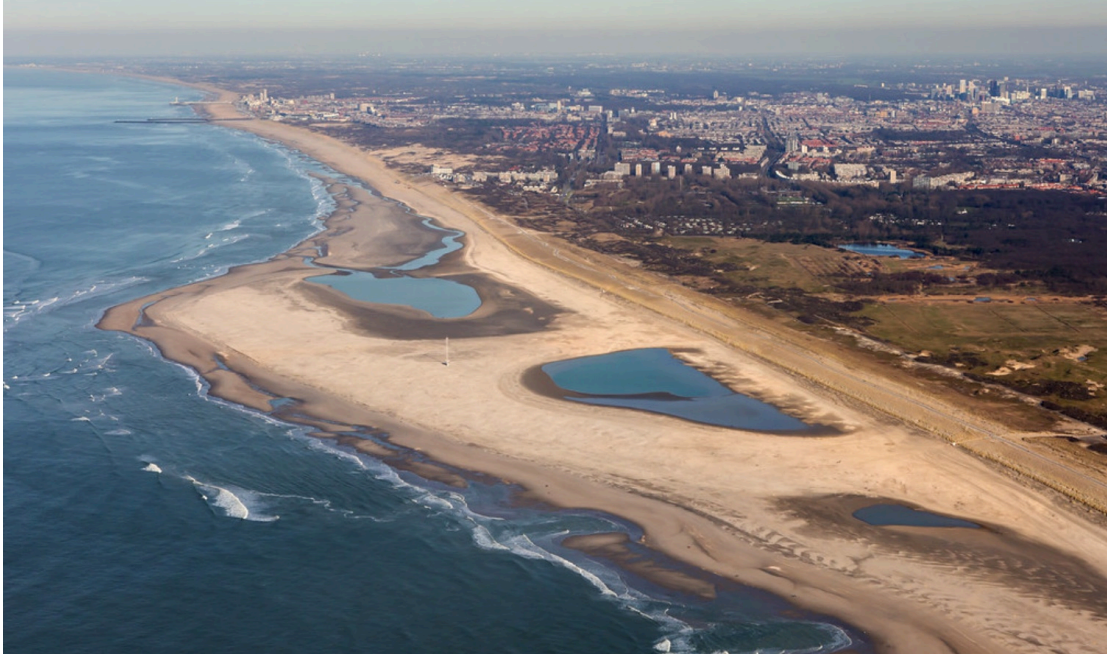
Fig. 15, Zandmotor (Sand Motor) in Rijkswaterstaat, Netherlands replenishes the beach from a single source of placed sand, negating the need for machine intensive replenishment projects, 2016 (Source: Jurriaan Brobbel)
