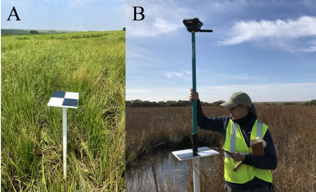
Figure S1. (A) Ground control point (GCP) deployed in the marsh and (B) surveying the GCP with an RTK GPS.
