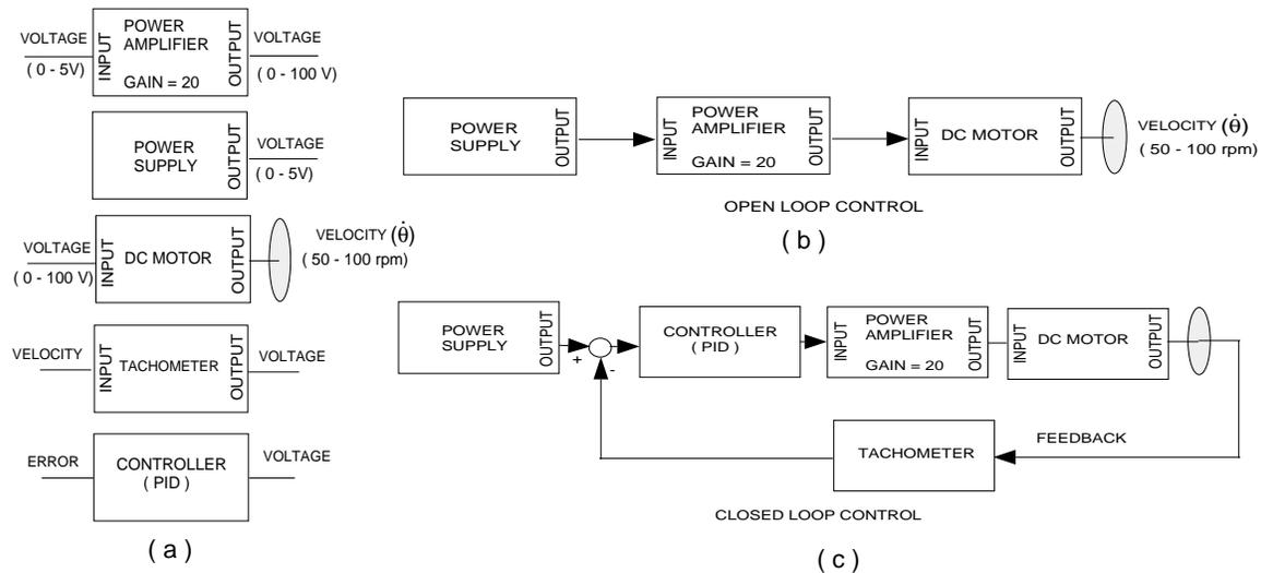
Figure 5: Figure 5: An example of a control system. (a) Components of the control system. (b) Open-loop control. (c) Closed-loop control.
