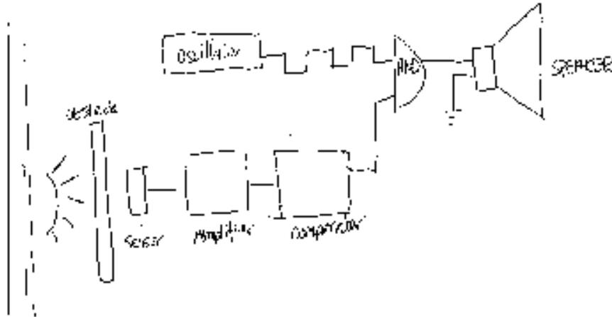
Figure 4: A student's understanding of the operation of the burglar alarm.
