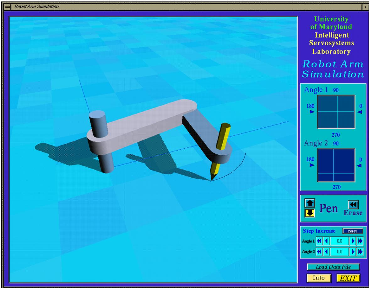
Figure 3: Simulation of Writing Instrument Manipulator.
