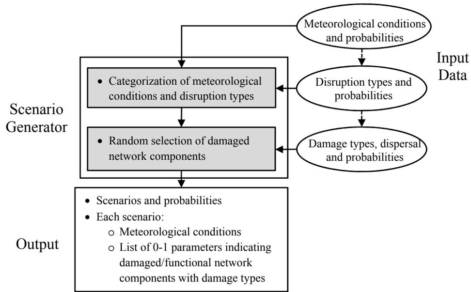
Figure 4-4 The flowchart of scenario generator
