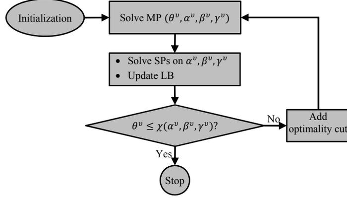
Figure 3-9 The general flowchart of Benders-based decomposition methods
