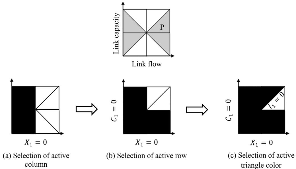
Figure 6-3 The schematic of the three-step process of active triangle selection in Vielma and Nemhauser (2011)'s logarithmic piecewise linearization method
