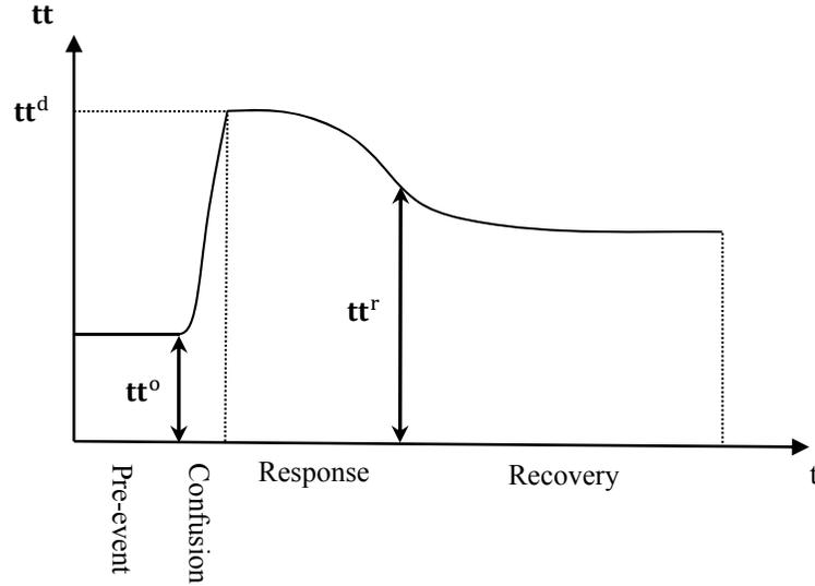
Figure 6-1 Travel time disruption profile for passenger traffic in a roadway network, where  $tt^0$ ,  $tt^d$ , and  $tt^r$  are the total travel times at the end of the pre-event, confusion, and response stages
