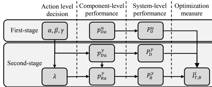
Figure 3-8 Schematic connecting IPP elements to its objective function
