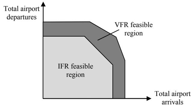
Figure 4-2 Typical airport-level capacity envelopes given runway configuration (FAA, 2004)
