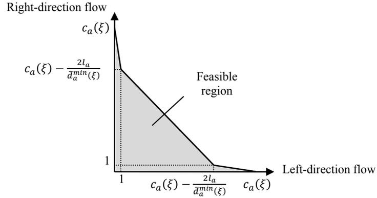
Figure 4-1 Directional capacity envelop in taxiways
