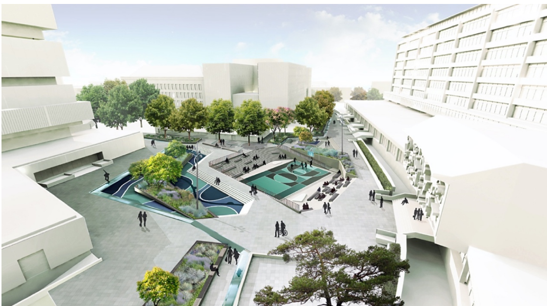
Figure 33: Water Squares in Rotterdam, the Netherlands double as functional public spaces and drainage infrastructure. Drawing attention to stormwater management in the public realm serves to educate the public. (Credit: De Urbanisten)
