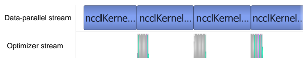
Figure 3.5: An Nsight profile of AxoNN training a 12 billion parameter transformer model on 48 GPUs shows the interleaving of the all-reduce and optimizer phases for a single batch. The two rows represent separate CUDA streams for the optimizer and all-reduce.
