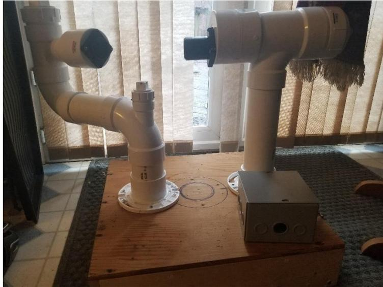
*Figure 33: Mechanical design of the 150ml sampling volume meter with movable detector, fixed laser, and electrical box.*
