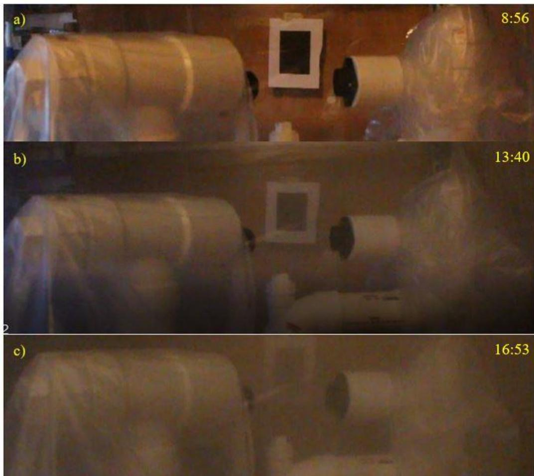
Figure 44: Frames saved from a video showing the change in the fog level over the first 25 minutes of data collection. This was taken on March 20<sup>th</sup>, 2019.
