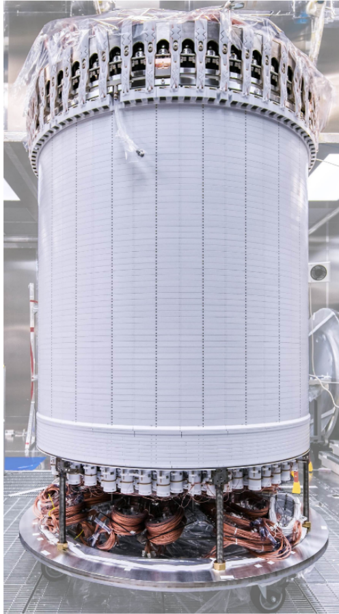
Figure 2.13: An image of the LZ TPC before being inserted in the inner cryovessel is shown. Some of the 93 top side skin PMTs can be seen above the PTFE, pointing downward in the ring lining the top of the field cage. The bottom dome skin PMTs are not visible but are assembled under the bottom PMT array (image from [32]).
