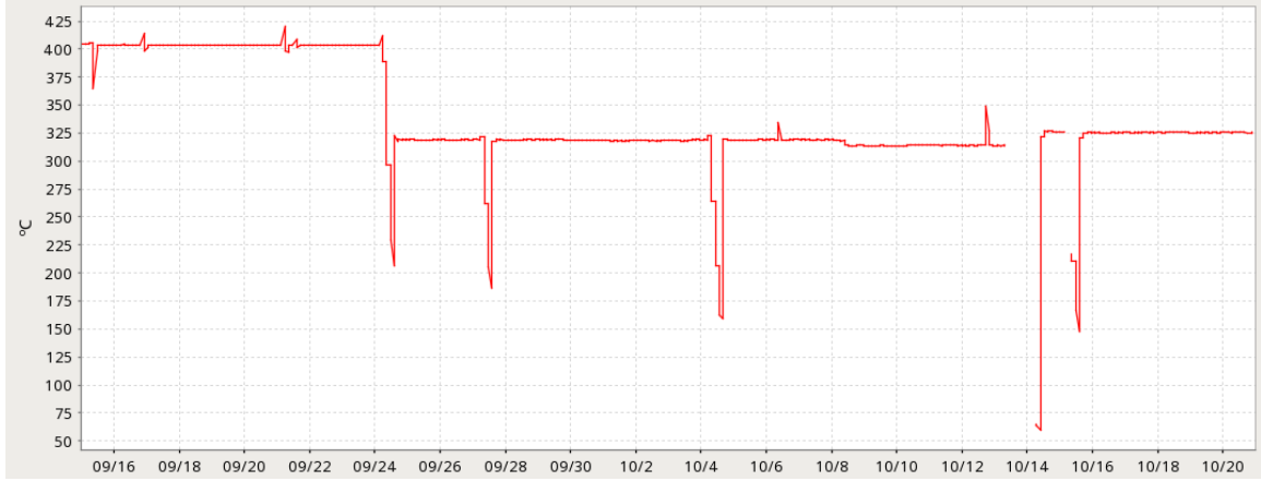
Figure 5.4: The getter temperature is shown before and during the October 2021 CH 4 removal test. The temperature fell below the nominal 400 °C operating temperature in late September 2021. Several minor disruptions to the circulation flow rate caused slight transients in the getter temperature prior to the test start, on the morning of October 6. The getter's steady state temperature dropped slightly when the flow rate was increased on October 8. There is a slight gap in the getter temperature data between a circulation stoppage and the flow rate reduction on October 14.
