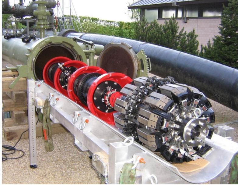
Figure 1.2: An example of a smart pig (in-line inspection device) [iecetech.org]
