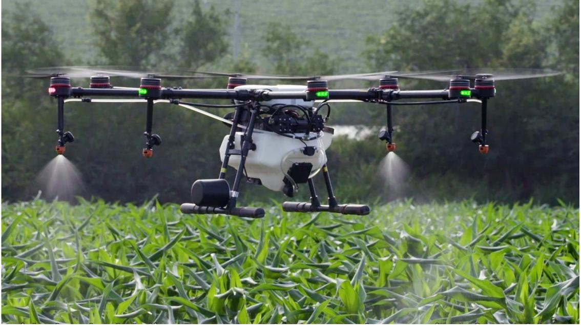
Figure 1.2: The MG-1S drone is seen spraying liquid into crop fields. Image retrieved as screen capture from <https://www.youtube.com/watch?v=P2YPG8P09JU> in June 2018.
