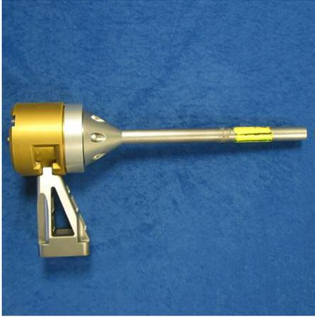
**Figure 5.1 Ranger Bare Bolt Drive Tool with tool post attached, from [34]**
