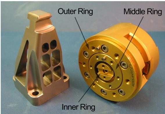
**Figure 2.5 IEEM and tool post disengaged, from [34]**
