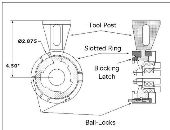
**Figure 2.4 IEEM locked to tool post, from [34]**
