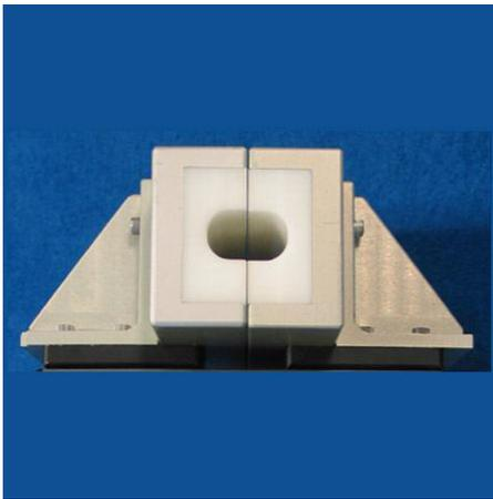
**Figure 5.2 Ranger EVA Handrail Gripper Fingers, from [34]**
