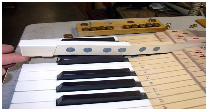
xvii. Photo of the weights embedded within a piano key
