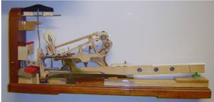
xvi.. Photo of the action of a single key
