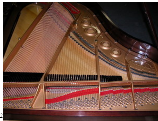
xix. Photos showing the similarity of the string lengths at the highest octave between pianos models
