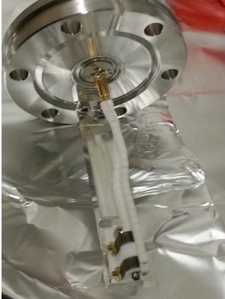
Figure 22: Room-temperature oven setup: The oven design is the same as in Fig. 20, but on a vacuum flange so it can be placed far from the 4K region.
