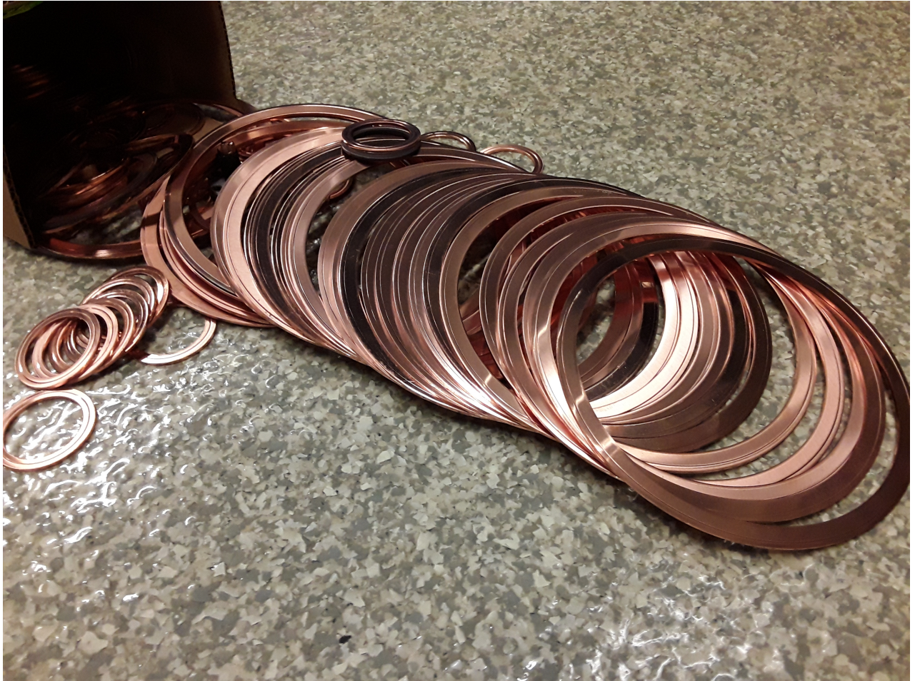
Figure 42: Copper gaskets used to seal the 8" vacuum flange: This collection of copper gaskets represents the number of times that the vacuum was opened and closed in the process of tuning the in-vacuum resonator, and make improvements inside the vacuum.
