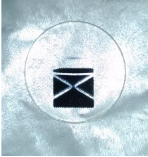
Figure 23: Negative of trap blades along axis of room-temperature oven : Accidentally, the room-temperature oven was on 9 Amps for about 10 minutes and the insides of the vacuum chamber became coated in Yb. Here is an artifact from this event.
