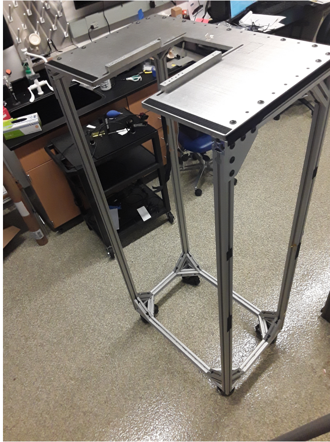
Figure 41: Service station: When the cryostat is removed from the experiment, it is placed in this 'service station'. Here, the vacuum cover and the radiation shields can be removed so work can be performed on the in-vacuum apparatus.
