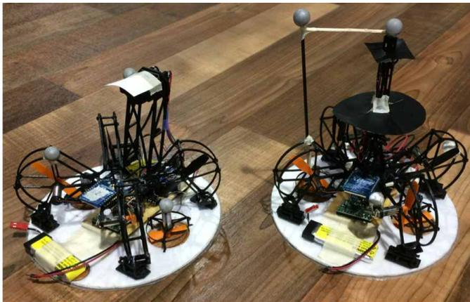
Figure 4.3: Autonomous pursuer hovercraft with onboard camera (left), and target hovercraft with IR light tower (right).
